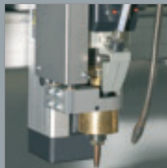
FSE Component Liquid spray unit to wet/spray the welding position before welding (pulse dosage)
